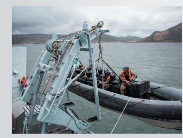
logistic support equipment needed for the boat. The complete system fits onto an ISO container footprint mounted and adapted on the ship's deck. The davit system can accommodate boats of various hull shapes weighing up to five tonnes. The boats and the crew can be lowered and retrieved safely by the davit system with the hosting ship underway. Two of these davit systems are normally fitted to a ship, with another two boats housed in the ship's boat bay on CSIR-developed cradle systems.
