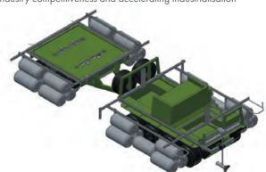
Geckos were fitted with flotation devices and additional propulsion so that they could go from the road into the water.
