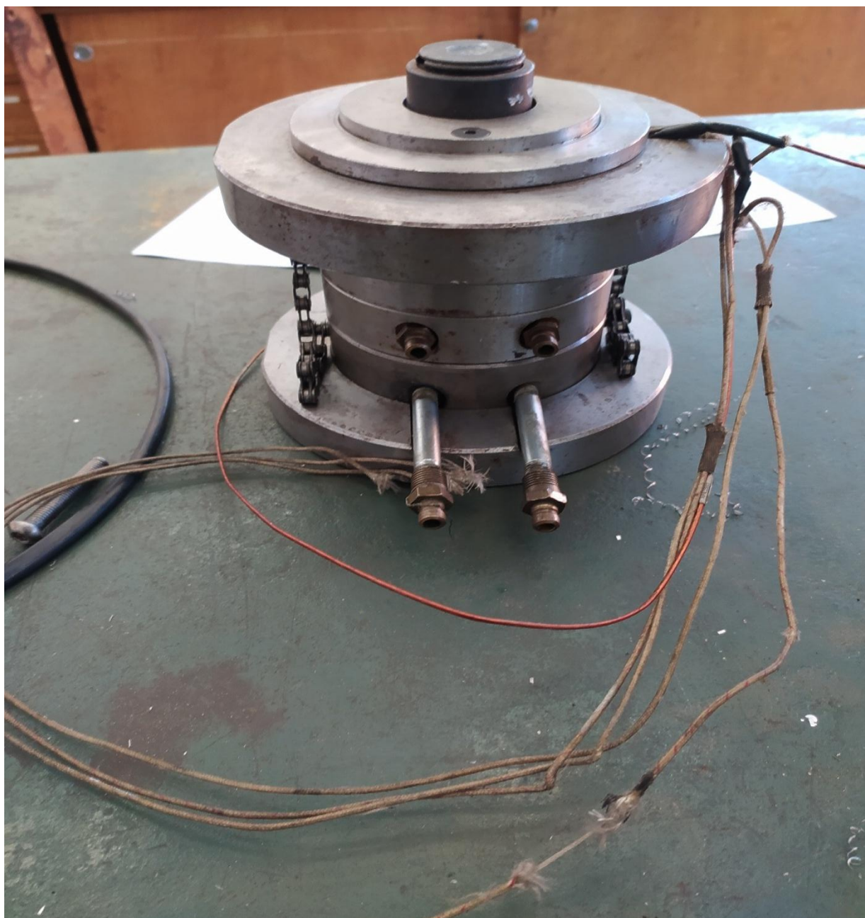
Fig 5: Transducer Nose mould for medical-grade injection-moulded part
