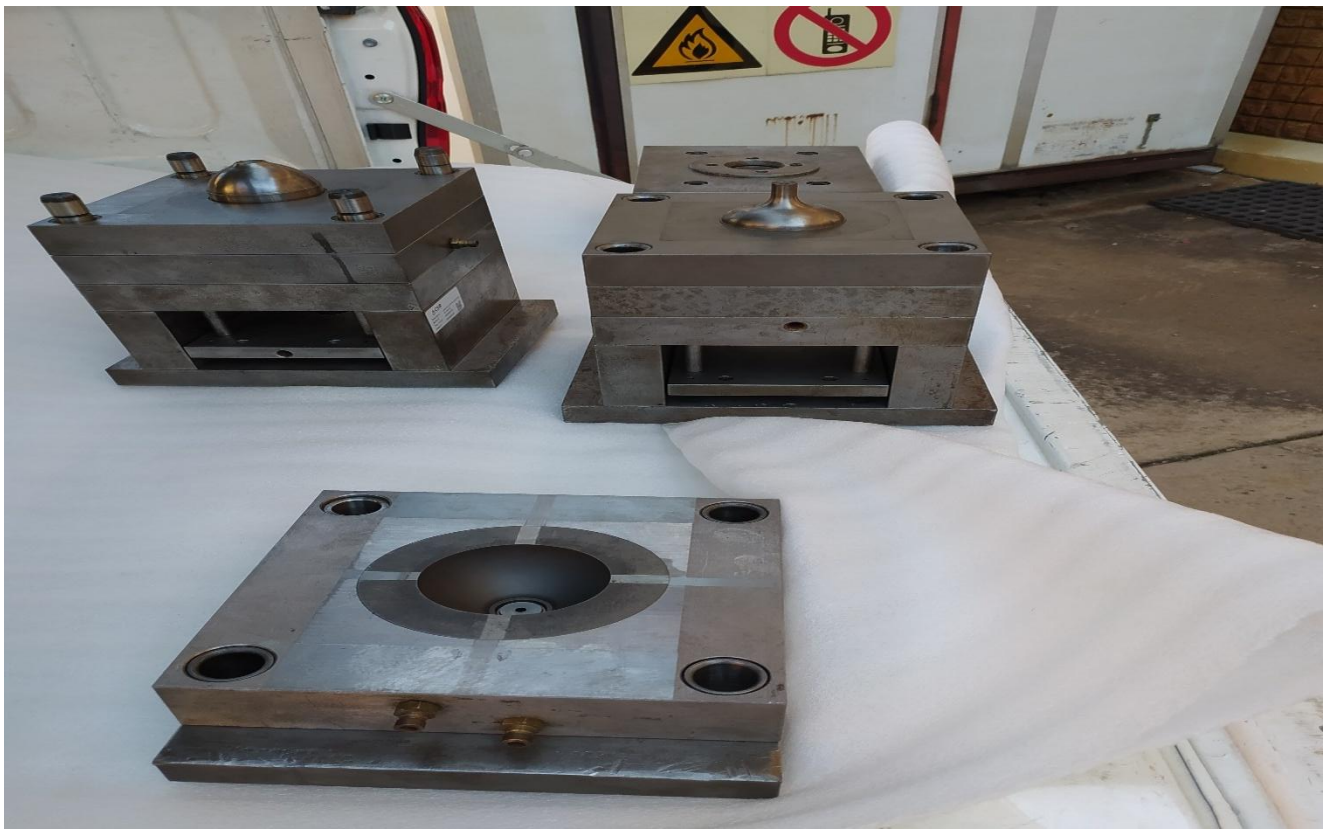
Figure 1: Upper mould for medical-grade injection-moulded part (RHS)
