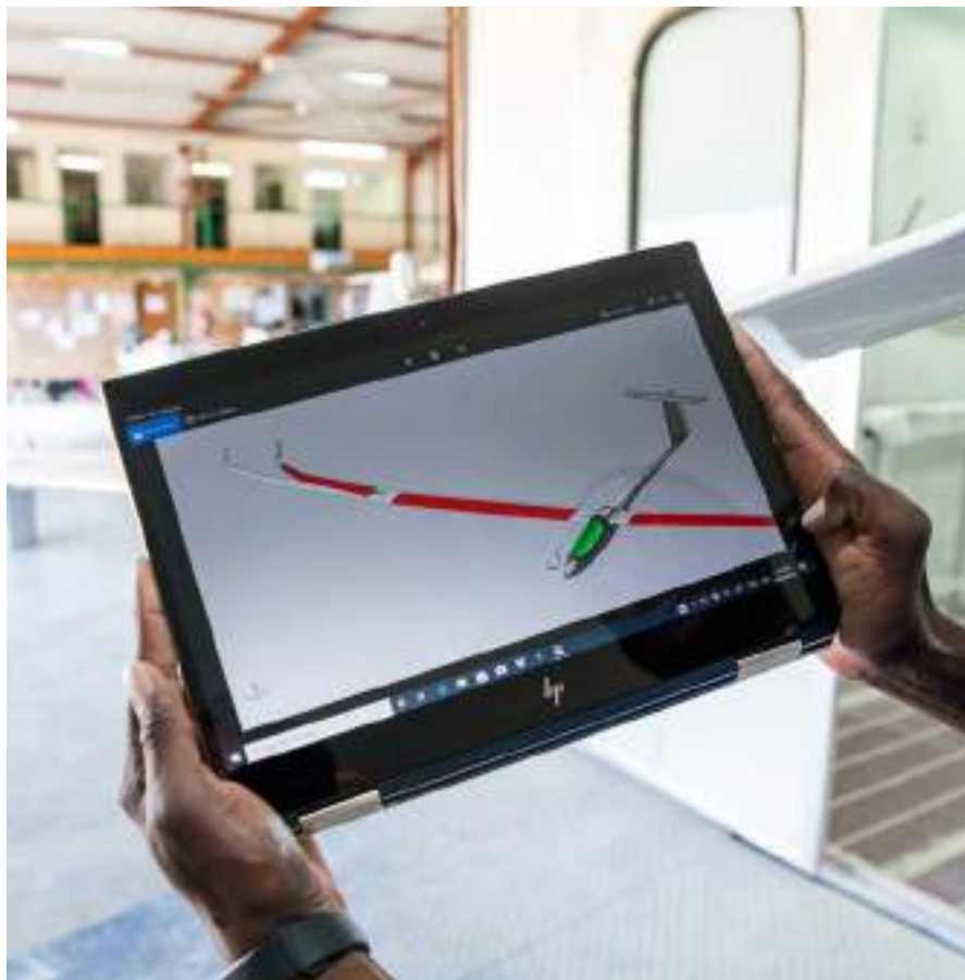
> A computer-aided design illustration of the extended wingspan from the current 21 m to the new 24 m.
