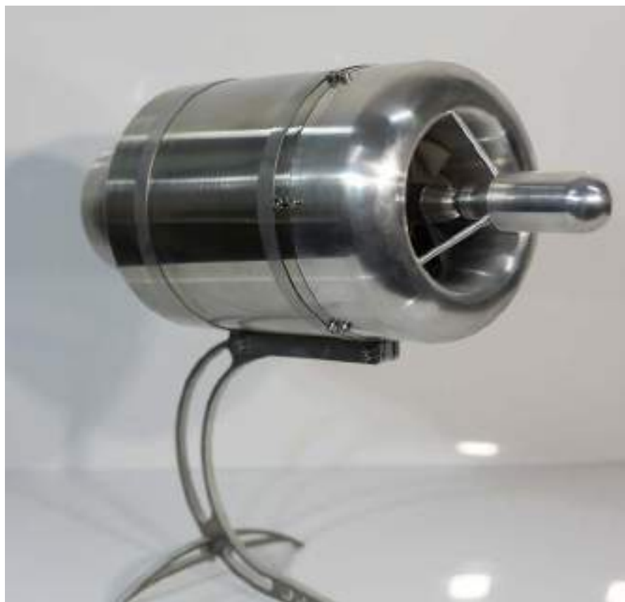
> The CAT 400 turbine, which produces 400 N thrust at sea-level static conditions.
