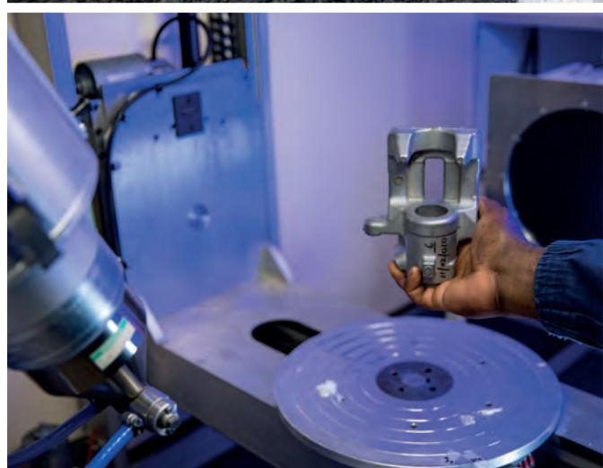
**H**ot Isostatic Pressing (HIP) is a specialised manufacturing process employed in industrial sectors to eliminate internal defects in components that occur during the initial manufacturing process. This is achieved by subjecting components to a blend of high temperature and high gas pressure (approx. 2000 bar) within a regulated environment
