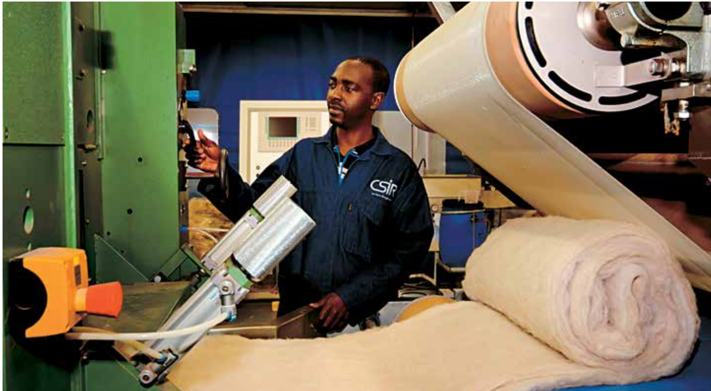
Dr Doice Moyo oversees the production of a novel thermal and sound-insulation material from waste products. The dual insulator mat is suitable for use in the building industry.
