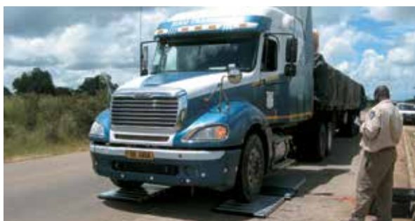
Staff at the Malawi Road Traffic Directorate undertake an axle load survey at Chileka on the road between Lilongwe and Mchinji on the border between Malawi and Zambia.
