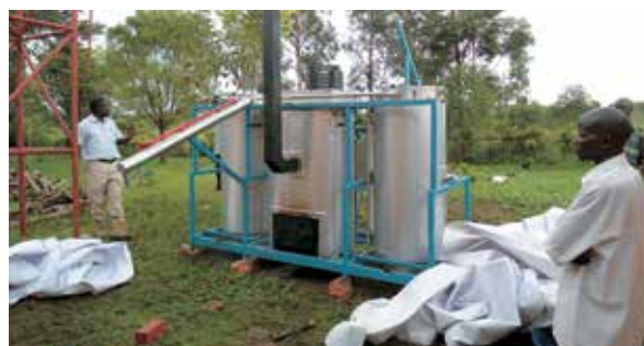
A distillation unit installed at the essential oil pilot project near Kampala, Uganda.
