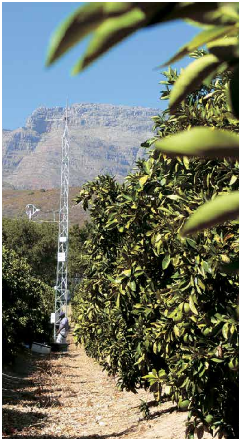
An Eddy Covariance system on a lattice mast in an orange orchard measures turbulent eddies of air above a vegetation canopy. These are important drivers of water vapour exchange from the underlying vegetation. Researchers use this and other equipment to measure the water use of fruit trees.
