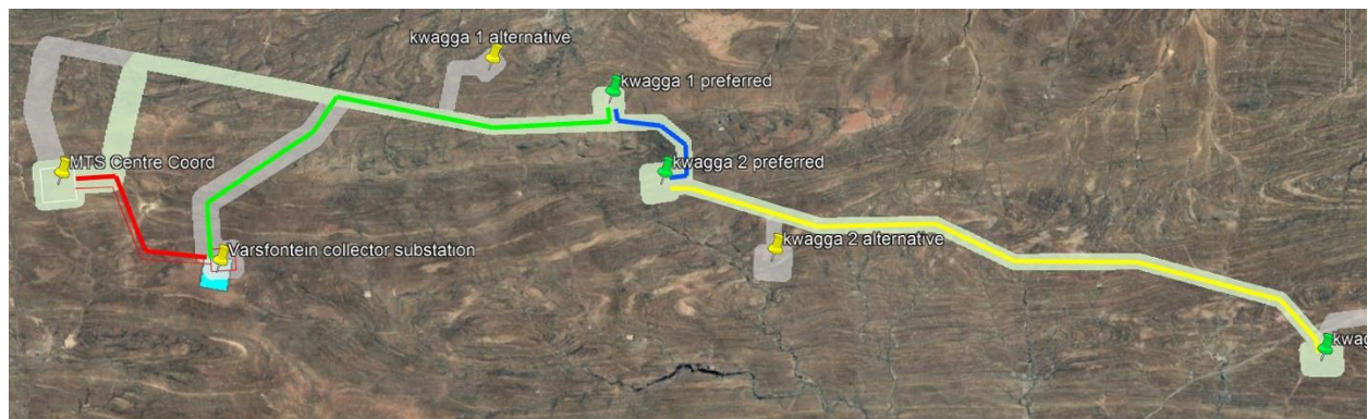
Figure 17: Location of Segment B – D (via C) (green and blue lines) along the Kwagga overhead transmission powerline route.
