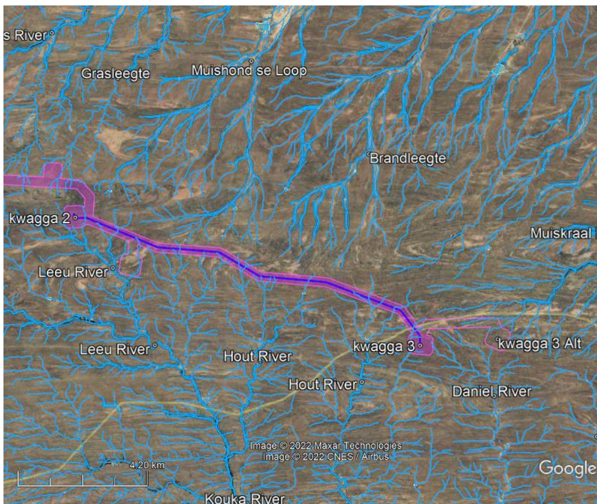
Google Earth image showing the layout for Section D to E of the proposed OHPL together with the mapped aquatic features
