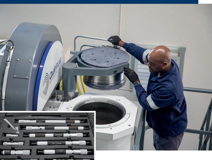
ot Isostatic Pressing (HIP) is a specialised manufacturing process employed in industrial sectors to eliminate internal defects in components that occur during the initial manufacturing process. This is achieved by subjecting components to a blend of high temperature and high gas pressure (approx. 2000 bar) within a regulated environment
