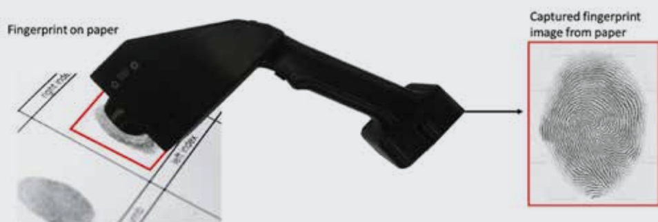
An illustration of the fingerprint device capturing a fingerprint from paper
