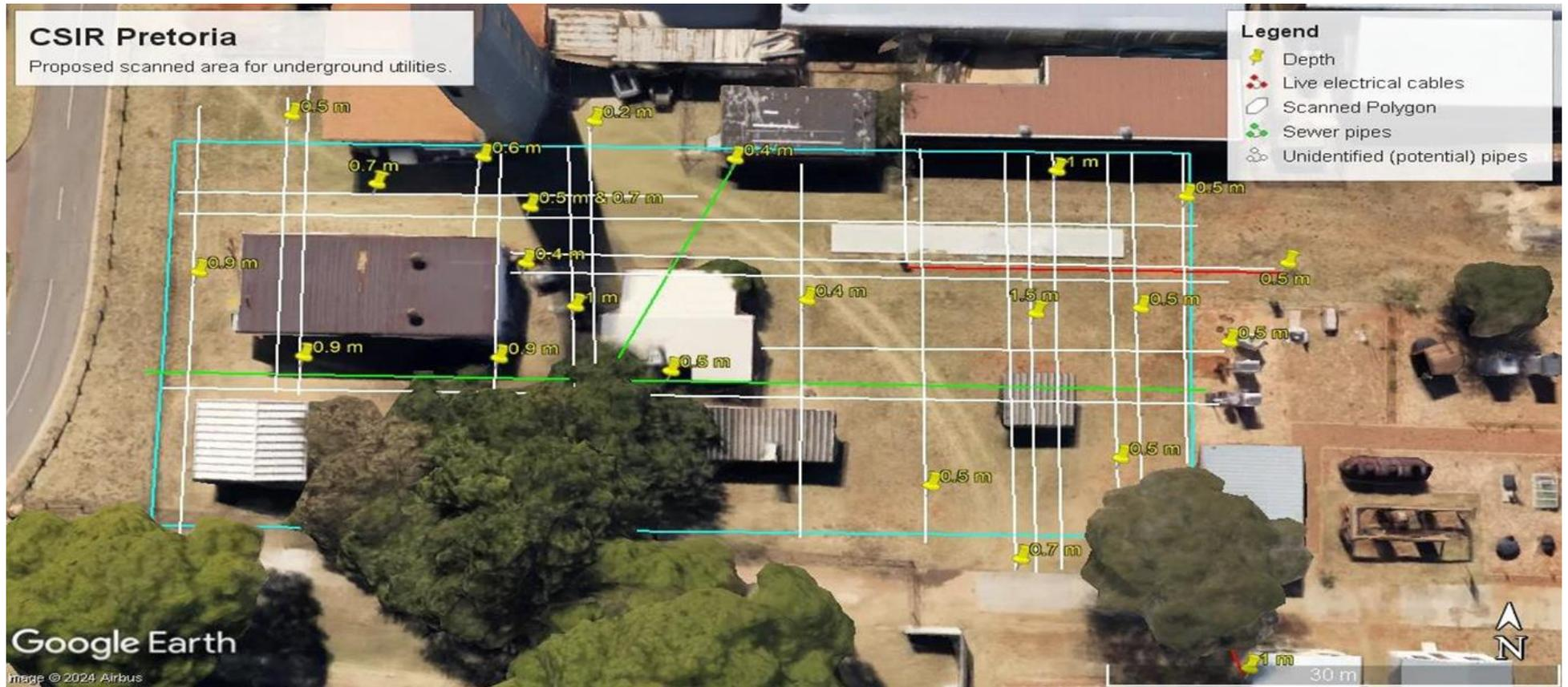
Figure 3. Satellite view of the scanned area and marked services, markings are not georeferenced.
