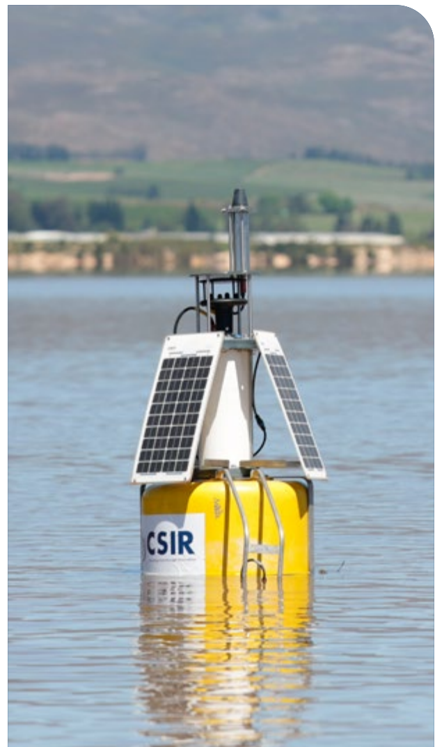
A buoy, equipped with a series of instruments for continuous data collection, in the Theewaterskloof Dam in the Western Cape. (Left) CSIR researchers deploy the buoy.
