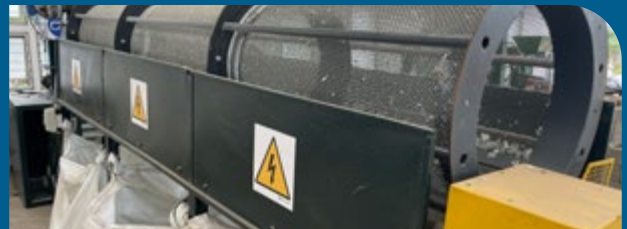
Glass collected by community members is crushed in a hammer mill. The aggregate is channelled through a rotating screen trommel to separate the different grades of recovered glass.
