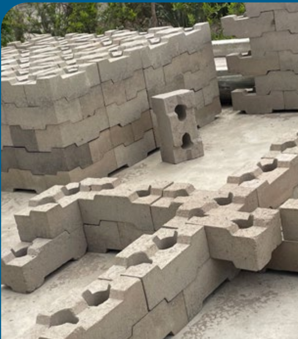
Up to 70% of the traditional raw materials in the new building block can be replaced by recyclable materials such as collected glass and construction waste.
