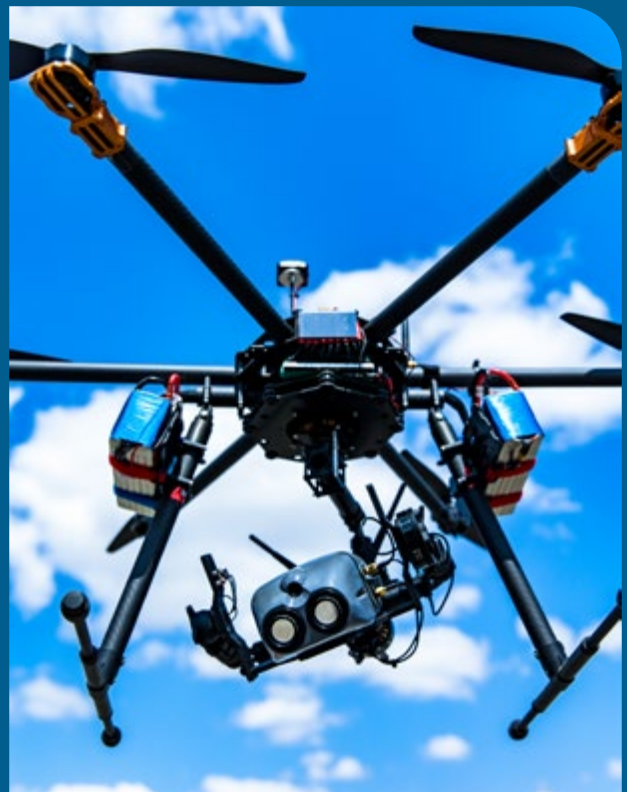
The CSIR K-line technology aboard an Autonosky drone to assist the Western Cape Fire Emergency Services with firefighting efforts.
