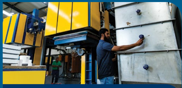
CSIR engineer Muhammad Sheik at CERadvance with a CSIR-developed thermal battery capable of storing waste heat and re-using it in the process when required.
