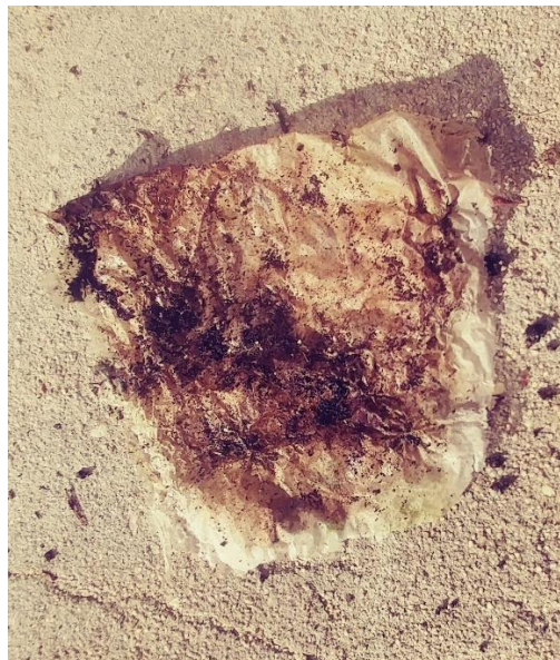
Figure 12: PE coated cup 4-6 years after disposal to a home composting system
