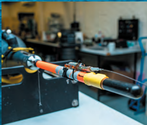
The antenna of an autonomous underwater vehicle being inspected by Sea Technology Services before deployment.
