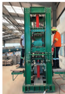
A prototype block machine with specialised moulds.
