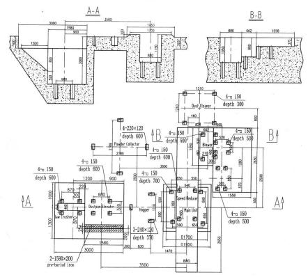
Note: the foundation of jaw crusher should be decided according to the machine model in the actual situation.
