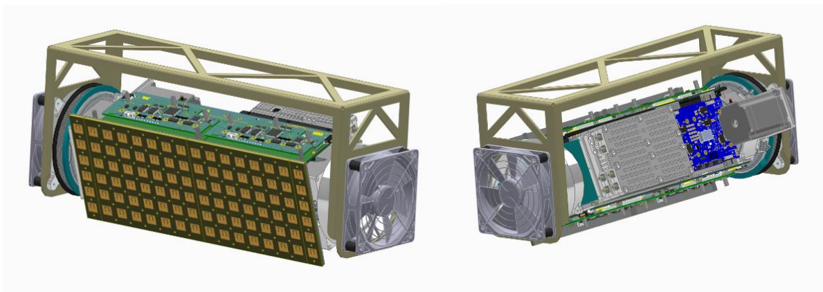
Payload approximate dimensions as it would typically be installed into the UAV
