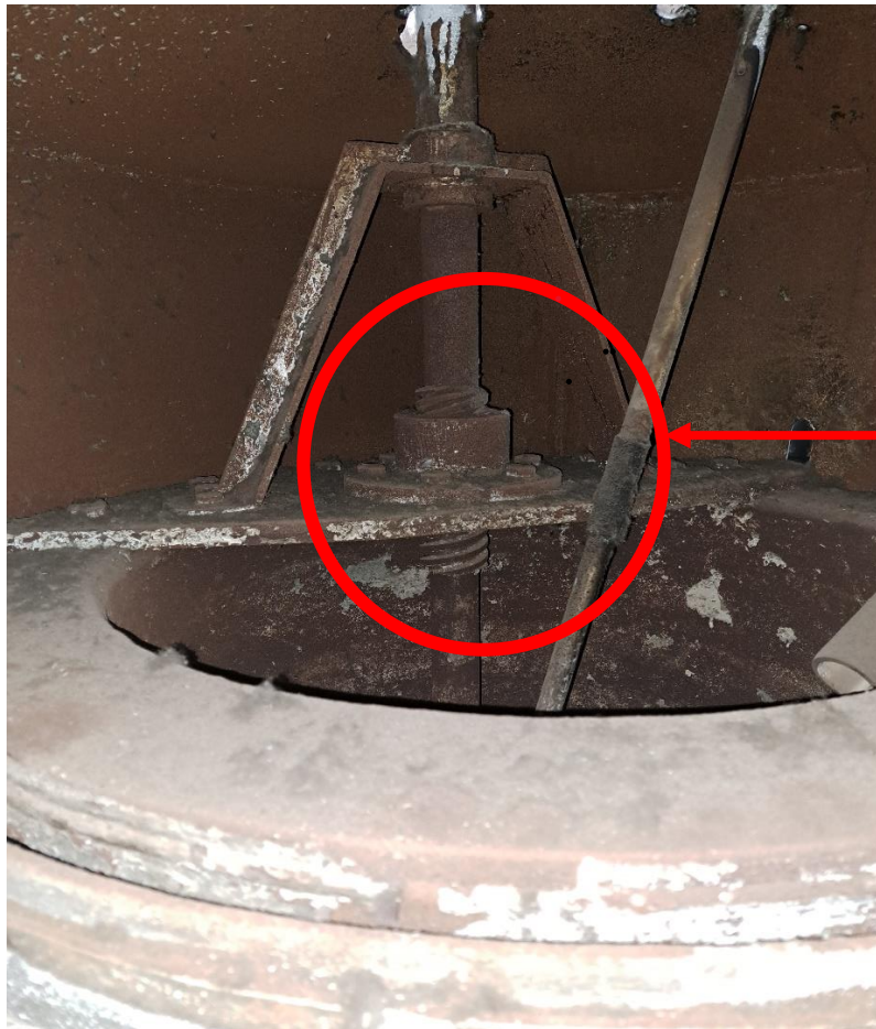
Fig 2: Screw type spout operating mechanism
