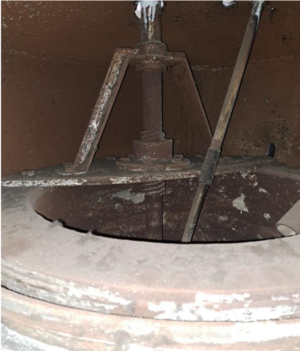
Figure 2: Screw type spout operating mechanism.
