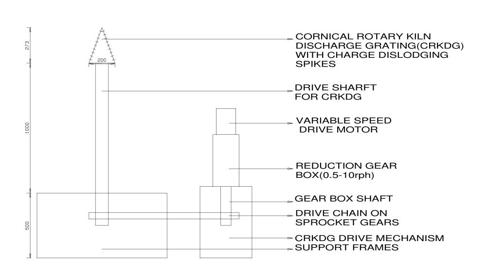
SECTION B-B: KILN DISCHARGE MECHANISM Drawing specifications:
