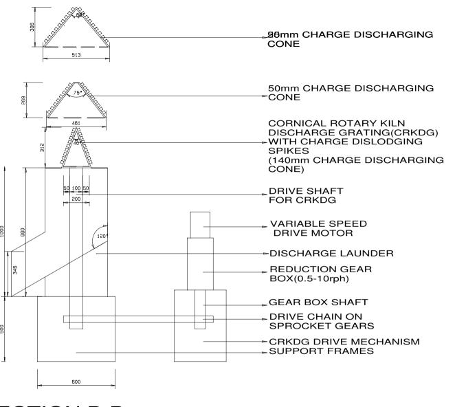
SECTION B-B: KILN DISCHARGE MECHANISM Drawing specifications
